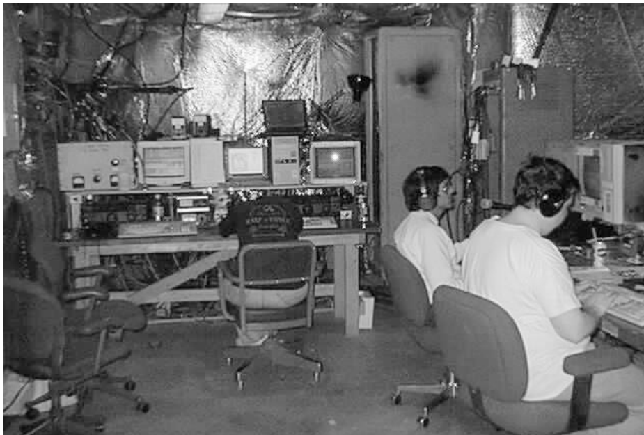
Two of the W3LPL operating positions - 20M on the left, 40M on the right. The rack in the background just to the right of center is the 4000V power supply that powers all six final amplifiers
