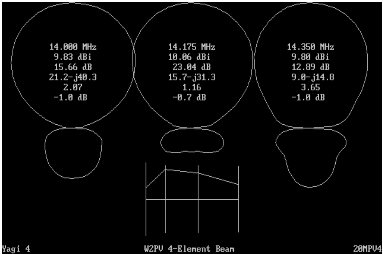
YO screen - W2PV 4, 40' boom
